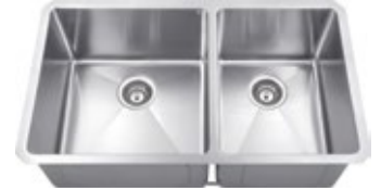
HMS260L - 16-Gauge Stainless Steel Undermount Sink with two unequal bowls 32" L x 19" W x 10-3/8" D Grid sold separately (HMS260-GRID) Strainer sold separately (STRAINER-200)
